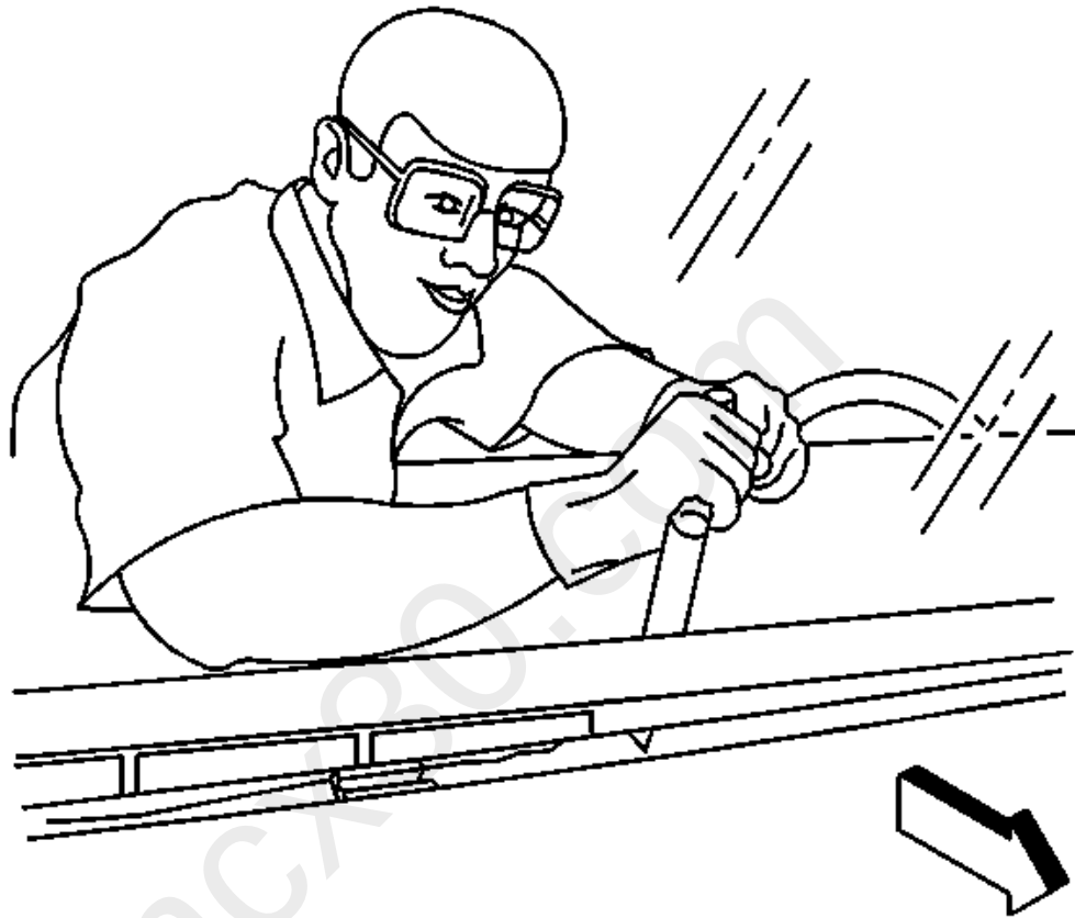
Fig. 10: Separating Bottom Of Window
